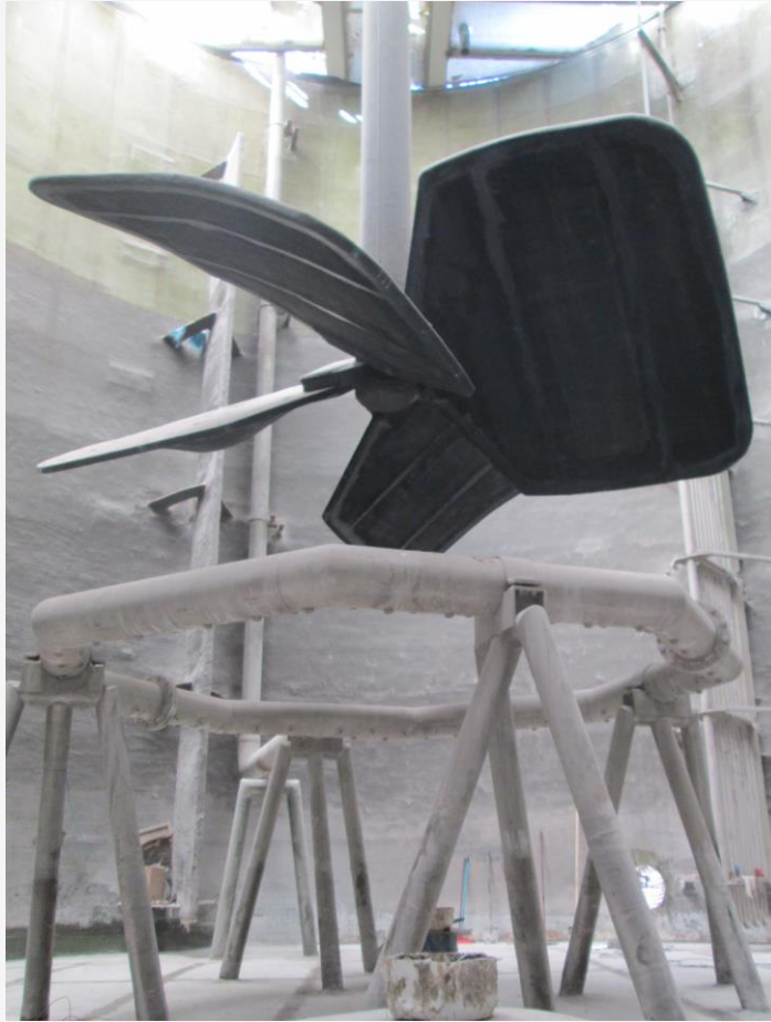
Bioleaching Copper Reactor 110kw, 5.8m dia
