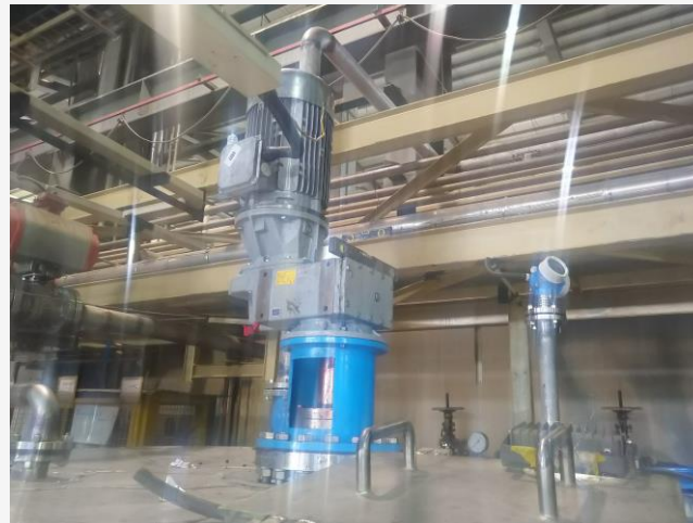
Copper Refinery Stripping Reactor 22kw, 1.8m dia
