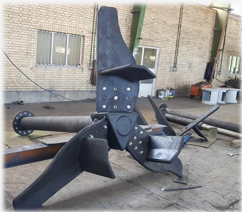
Iron Ore Concentrated Agitator, 55kw, 2.5m dia
